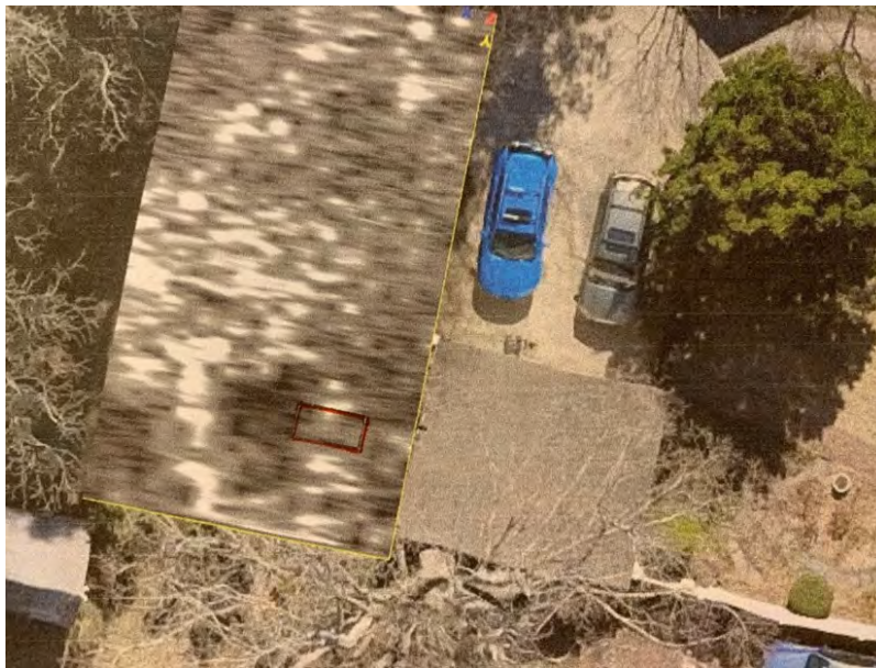
Aerial photo showing the GPR scan on the left at a depth of 1.5m with the trench location in red, and on the right the garage, with the cars waiting patiently outside.
